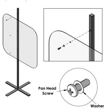
**STEP 7:** Use screwdriver to tighten screw to Metal Upright. Repeat above steps for remaining two holes to fully secure Divider Panel to Metal Upright.
