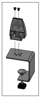
**NOTE:** There are multiple hole locations in top of C-Clamp Base. Please use highlighted holes when mounting Clamp Back to C-Clamp Base.
