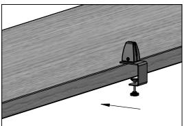
**STEP 7:** Repeat STEP 6 to install your other assembled Clamp on opposite side of Bar/table.
