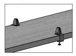
**STEP 9:** While one person supports the Divider Panel, have the other person use supplied Hex Key to tighten Hex screws in Clamps until Panel is snug.
