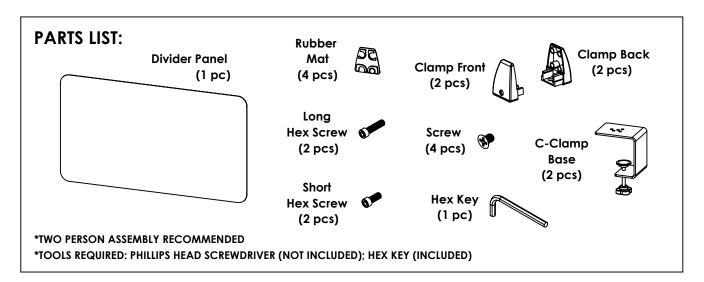
**STEP 1:** Insert Rubber Mats into Clamp Fronts and Clamp Backs.
