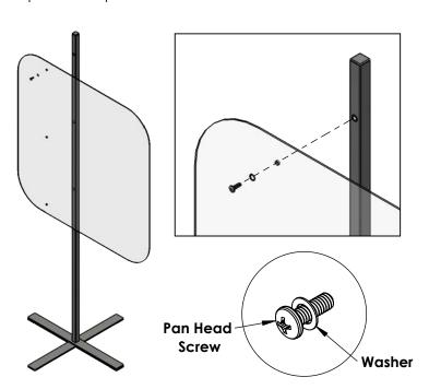
**STEP 7:** Use screwdriver to tighten screw to Metal Upright. Repeat above steps for remaining two holes to fully secure Divider Panel to Metal Upright.
