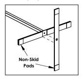
NOTE: Countersunk Hole on bottom of Leg Brace should be facing out
