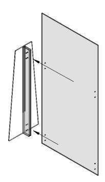
**STEP 3:** Insert one of the provided Screws through hole in Side Channel Upright. Guide it through hole in Main Panel and out the other side of channel.
