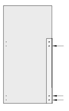
**STEP 6:** Stand up remaining Side Channel Upright and guide other side of Main Panel Upright into channel, again making sure holes are aligned. Repeat Steps 3-5 to secure Side Upright to Main Panel.
