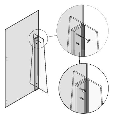
**STEP 5:** Repeat Steps 3 & 4 for remaining 3 hole locations on that side of Shield.
