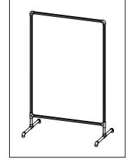
**STEP 10:** Stand assembled unit upright on flat surface and make sure all connection points fit snugly together.
