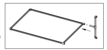
Connect remaining Foot Subassembly into open end of Tee fitting
