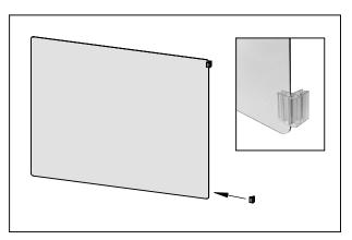
**STEP 5:** Repeat STEPS 2 - 4 to install remaining four L-connectors on opposite side edge of Front Panel.
