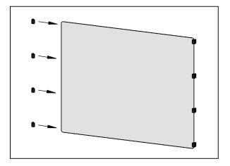
**STEP 6:** Take one of the Side Panel subassemblies and attach it to one side of the Front Panel by pushing into installed L-connectors on Front Panel.
