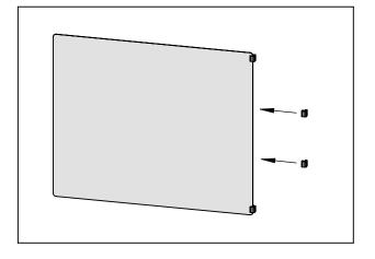
**STEP 3:** Take another L-connector and push onto the side edge of Panel at bottom, just above rounded corner.
