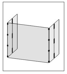
**STEP 8:** Use the adhesive-backed T Shaped Gripper Connectors (included) to attach barrier securely to desktop. Install one in the middle of the bottom edge of each Side Panel and two additional ones evenly spaced on the bottom edge of the Front Panel.
