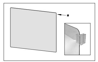
**STEP 4:** Add two additional L-connectors to side edge of Front Panel, evenly spaced out between installed L-connectors (~ 8" apart).
