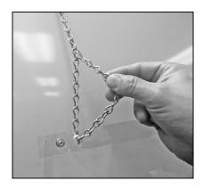
STEP 7: Repeat STEP 6 for attaching right chain through hole in top right of your clear Vinyl Shield.
