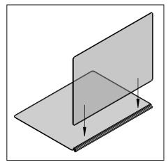
**STEP 4:** Stand assembled panels upright on flat surface. Insert another clear panel into one of the open slots in X-Connector. Start by angling the top part of panel into X-connector, then push bottom corner into bottom of connector. Lastly, push the long edge of panel firmly towards X-connector and make sure panel is fully engaged with channel in X-connector.
