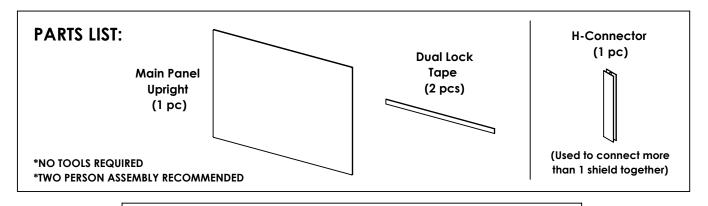
NOTE: Prior to mounting Shield, clean the area where the Dual Lock tape will be applied with a 50/50 mixture of isopropyl alcohol (IPA) and water for proper adhesion.
