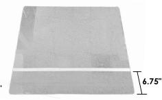
To achieve a min shield height of 16" above mounting surface, apply the Dual Lock tape 6.75" from the bottom edge of the Main Panel Upright.
