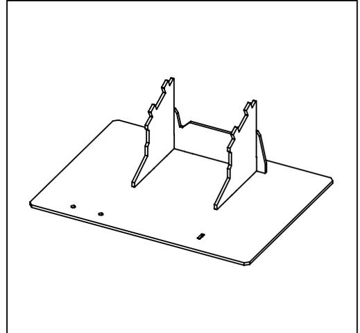
**STEP 4:** Insert Front Stand into Vertical slot at front of Base Panel (where applicable)
