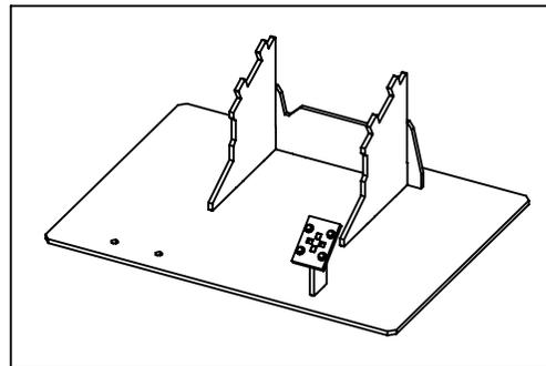
**STEP 3:** Use even pressure to insert LEGO® Studs into hole cutouts on Base Panel where applicable.
