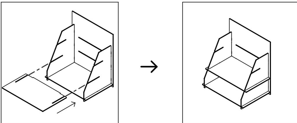
**STEP 5:** Insert the Top Panel into the top slot of each Side Panel, as shown below. Ensure tab on rear of panel is inserted into slot on Back Panel.
