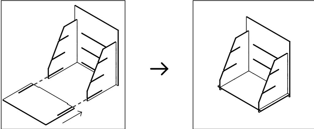
**STEP 4:** Insert the Middle Panel into the middle slot of each Side Panel, as shown below. Ensure tab on rear of panel is inserted into slot on Back Panel.
