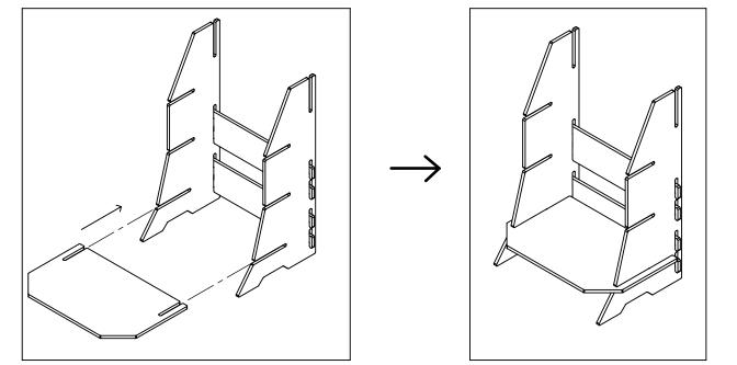
**STEP 4:** Take a Shelf and slide into the next slot opening from the bottom on the Side Panels. *Note: If needed, using a rubber mallet (sold separately), gently tap the parts into place .*
