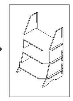
**STEP 6:** Insert remaining Header Shelf into top vertical slots on both Side Panels, as shown below. *Note: If needed, using a rubber mallet (sold separately), gently tap the parts into place .*
